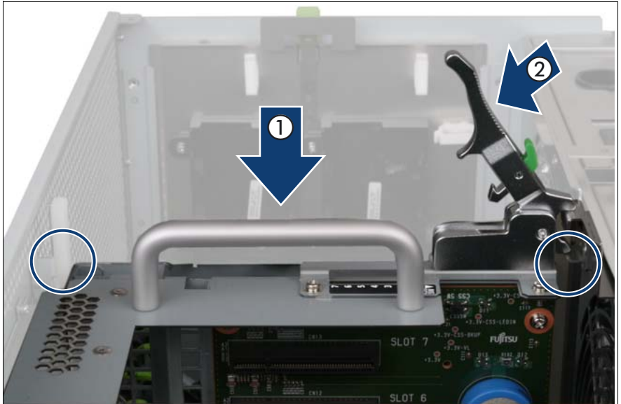
Figure 85: Installing the PCI Riser
